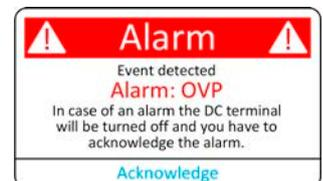
In order to acknowledge an alarm during analog remote control refer to “3.5.4.2. Acknowledging device alarms”. To acknowledge in digital remote control, refer to the external documentation “Programming Guide ModBus & SCPI”.
