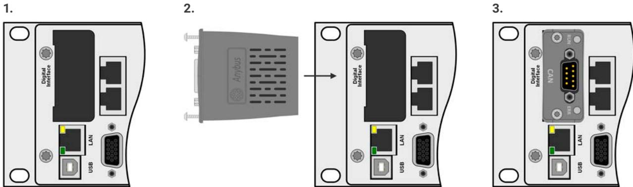
1. Remove the slot cover. If needed, use a screw driver.
