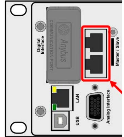
Figure 7 - Master slave bus ports
