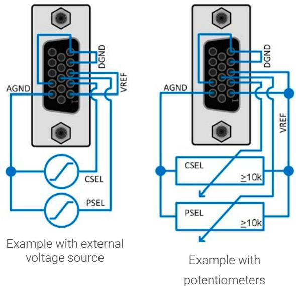
**!** When using the voltage range 0...5 V the effective resolution of set values and actual values halves.
