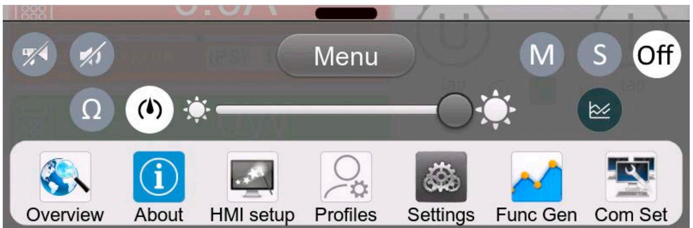
Tapping a button activates or deactivates the feature. Buttons with black on white indicate an activated feature:
