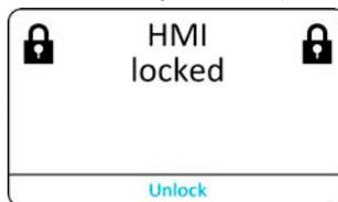
3. Unlock the HMI by tapping on **Unlock** within 5 seconds, otherwise the pop-up will disappear and the HMI remains locked. In case the additional PIN code lock has been activated in the **Lock** screen, another requester will pop up, asking you to enter the PIN before it finally unlocks the HMI.
