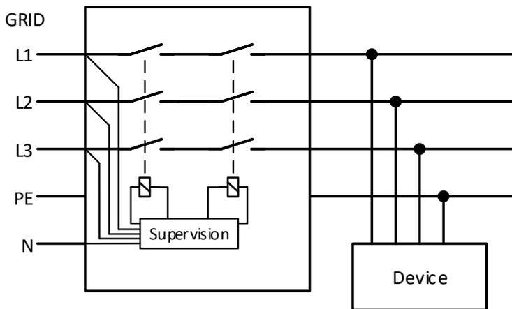
Figure 9 - Principle of an NS protection network
