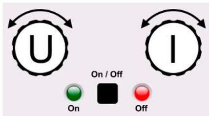
The physical quantities on the depiction of the knob show the current assignment. The left knob is always assigned to the voltage (U), while the right knob can be switched by tapping on the depiction. Furthermore, the DC input status is indicated by two LEDs (green = on).
