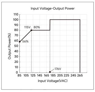
Note: For input voltage 85-115VAC, the input voltage should be derated based on the temperature derating.
