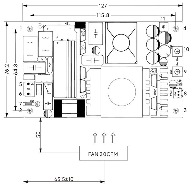
The cooling fan should blow air directly towards the power supply from the side or the top, as shown.
