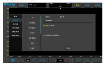
Select the respective test item, follow the description to connect wires, click OK and the oscilloscope will automatically configure the corresponding tests, easily solving most common issues encountered by automotive engineers.
