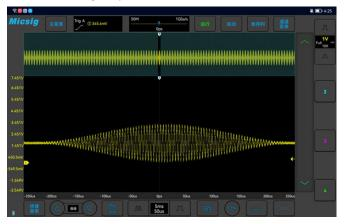
Memory depth up to 50Mpts, with Zoom technology, both the overall picture and details can be perfectly displayed.
