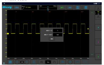
Helps measure the timing of the cyclic waveform. Set the cylinders number and angle, with the phase start and end points indicated by solid lines. Two phase scales can be dragged to appropriate positions to mark the start and end points of the cycle.
