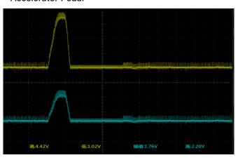
The accelerator pedal is the signal from accelerator. Generally, there are two sets, each with 3 wires: power, signal, and ground. They can be classified as analog/analog or analog/digital signals. Analog/analog signals consist of 2 analog signals, typically in two modes: a divergent signal and a convergent signal.
