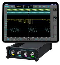
With the USB type-c interface, it can be used with any Android platform or device. Such as smartphones, tablet devices or Android-based computers.
