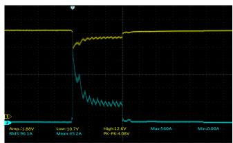
Use VATO with a current probe to conduct current testing during the starting process of a vehicle (both gasoline and diesel vehicles), able to observe whether the current waveform is normal or not.
