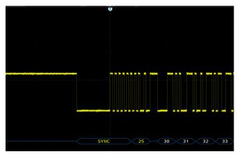
The LIN bus communication is widely used in automobiles, with low speed and the ability to connect multiple control devices on a single network. It can control non-safety-critical components of the vehicle at low speeds, such as wipers, windows, mirrors, air conditioning, and electronic seats.
