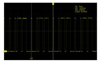
The camshaft position sensor is generally used for timing and is often tested in conjunction with the crankshaft sensor to determine the vehicle's timing. Common vehicle models have one or two camshaft position sensors, while it is less common to have four. Common types of camshaft position sensors include Hall-effect, inductive, and AC reluctance sensors.
