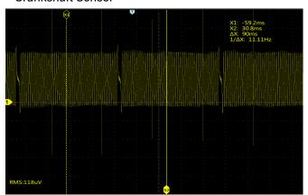
The crankshaft position sensor can be installed in various locations, such as near the front crank pulley or on the rear flywheel. The ECM uses its output signal to determine the precise position of the engine's crankshaft. Typically, there are two types: inductive and Hall-effect sensors.
