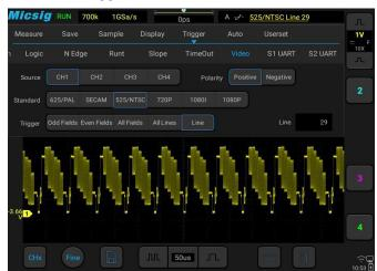
Support Edge, Pulse, Logic, N Edge, Runt, Slope, Timeout, Video and Serial trigger, most intuitive trigger settings.
