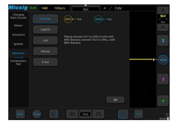
SATO is capable of acquiring and decoding CAN High /CAN Low, CAN FD, LIN, FlexRay, and K line signals, delivers professional Network communication tests on vehicles.
