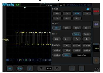
Support RS-232/422/485/UART, LIN, CAN, CAN FD,  $\rm l^2C$ , SPI serial bus decoding and triggering options, display waveform and data at the same time.
