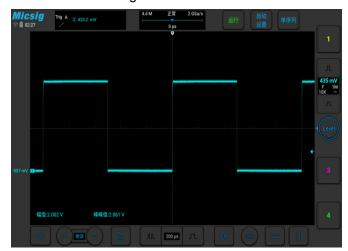
By pinching two fingers apart on the screen, you can adjust the vertical scale as you like, no longer limited by the 1/2/5 step limit.
