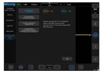
The electronic faults can be complicated, by comparing the collected various waveforms, users judgefaults by analyzing the timing and quantitative relationships between waveforms.
