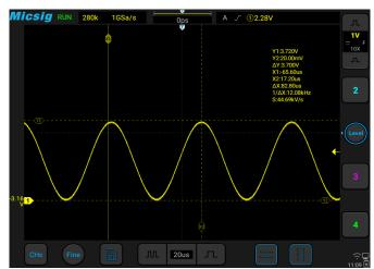
One touch to open horizontal and vertical cursors, each cursor can be moved separately or simultaneously.
