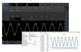
Users can save waveforms and measurement results as binary (BIN) or CSV format files for data analysis using Matlab or Excel. Also support saved as WAV format, direct open & analysis inside the oscilloscope. Additionally, user can save waveforms as images or record videos.
