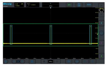
Traditional Single acquisitions can only capture signals continuously, wasted storage depth when testing intermittent signals like laser pulses or serial buses, also difficult to trace back captured events. While the segmented storage acquisition can capture the target signal and allows to play back captured ones, effectively captures target signals multiple times over a long period of time.
