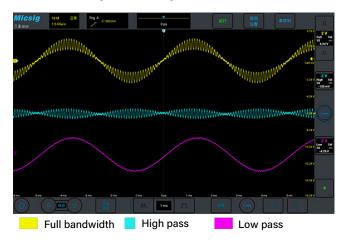
Digital filtering can selectively allow or block signal components within specific frequency ranges.
