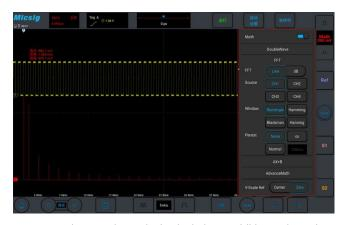
Support various mathematical calculations: addition, subtraction, multiplication, division, integration, differentiation, etc. Support custom function formula for advanced signal analysis. Also support FFT (Fast Fourier Transform) for real-time spectral analysis of collected waveform signals.
