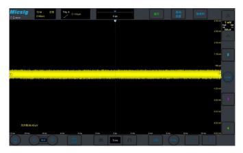
Even at its full bandwidth of 500M, the noise floor of the ETO still less than  $90\mu Vrms$ , allow engineers accurately capture weak but important signals during daily circuit debugging and signal analysis.
