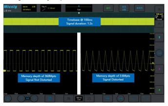
Insufficient memory depth often leads to distortion when long time base signals are expanded. With memory depth of up to 360Mpts, there is no reduction in performance even with two channels opened at the same time. The signals will still maintain excellent fidelity even at long time base.
