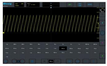
Traditional oscilloscopes need to step in a sequential manner when adjusting the time base. In addition to traditional sequential steps, the ETO series also has a time base matrix, allows user to reach any time base in one click.
