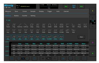
Simultaneously calculate the average, maximum, minimum, and root mean square of 10 measurement items, with a max count of up to 10,000, every waveform data is accurately recorded, provide more accurate and comprehensive readings.
