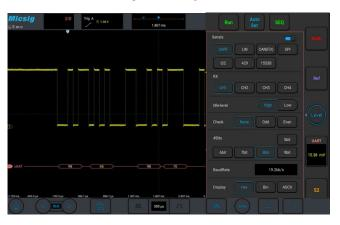
The ETO comes standard with 8 types of serial bus decodes: RS-232/422/485/ UART, CAN, LIN, CAN FD, SPI, I2C, ARINC429, 1553B. With the TXT decoding text mode, the data can be transferred to CSV format.
