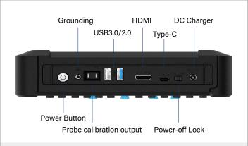
Power button, Grounding plug, Probe Calibration Output, USB3.0/2.0, HDMI, Type-C, Power Supply, Power-off Lock (Note: switch to ON for first-time use)
