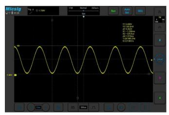
One touch to open horizontal and vertical cursors, each cursor can be moved separately or simultaneously, brings unmatched user experience.
