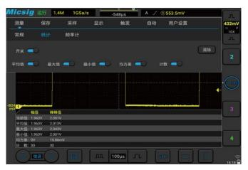
Using statistics to read the current measurement item multiple times, monitor the change trend, the maximum number of readings can reach 10,000.
