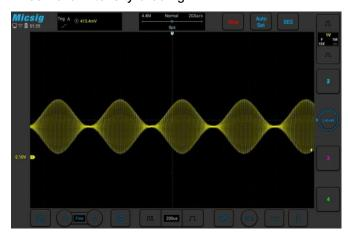
The TO series has digital fluorescent display, the resulting intensity-graded trace is brighter for events that occur with more frequency and dims when the events occur with less frequency
