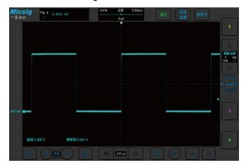
By pinching two fingers apart on the screen, you can adjust the vertical scale as you like, no longer limited by the 1/2/5 step limit.
