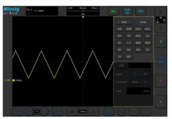
Users can set different labels for different sources to facilitate observation and readout.
