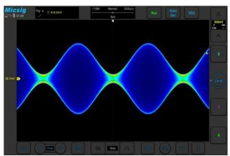
The Color temperature display is similar to the intensity-graded trace function, but the trace occurrence is represented by different colors as opposed to changes in the intensity of one color. Red colors represent more frequently occurred events, while the bule represents less frequently ones.
