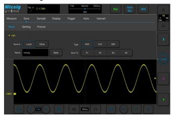
Micsig's unique fast storage function allow users quickly save waveforms with one press, a full screen of 220M waveform data can be completely saved in BIN format. More than 70% faster than traditional oscilloscopes.
