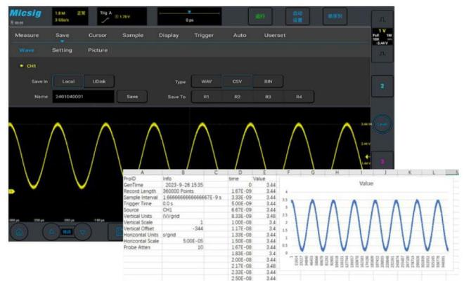
Users can save waveforms and measurement results as binary (BIN) or CSV format files for data analysis using Matlab or Excel. Also support saved as WAV format, open & analysis inside the oscilloscope. Additionally, user can save waveforms as images or record videos.
