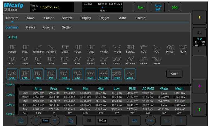
Simultaneously calculate the average, maximum, minimum, and root mean square of 10 measurement items, with a max count of up to 10,000, every waveform data is accurately recorded, provide more accurate and comprehensive readings.
