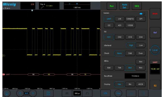
The MDO series is standard with RS-232/422/485/ UART, CAN, LIN, CAN FD, SPI, I2C, ARINC-429, 1553B. With the TXT decoding text mode, the data can be transferred to CSV format.
