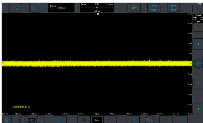
Even at its full bandwidth of 500M, the noise floor of the MDO series still less than 90µVrms, allow engineers accurately capture weak but important signals during daily debugging and signal analysis.
