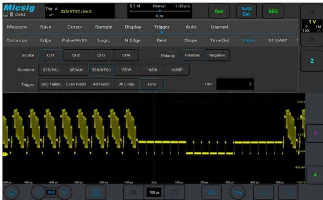
The MDO series provide multiple triggers, including edge, pulse width, logic, Nth edge, Runt, slope, bus decoding, etc. Whether you need to capture specific edge transitions, or observe duration and frequency of the target signal, it meets your requirement at ease.
