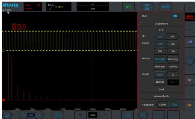
Support various mathematical calculations: addition, subtraction, multiplication, division, integration, differentiation, etc. Support custom function formula for advanced signal analysis. Also support FFT (Fast Fourier Transform) for real-time spectral analysis of collected waveform signals.
