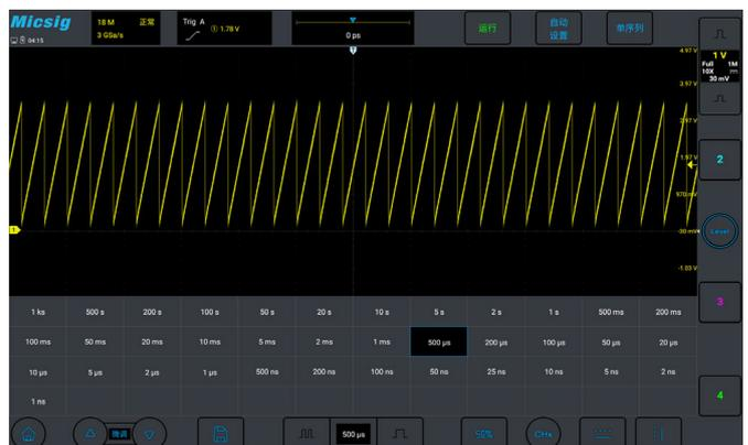
Traditional oscilloscopes need to step in a sequential manner when adjusting the time base. In addition to traditional sequential steps, the MDO series also has a time base matrix, allows user to select any time base in one click.
