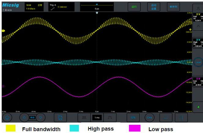
Hardware digital filtering can effectively filter out interference and noise, improve signal accuracy. Digital filtering can selectively pass or block signal components within a specific frequency range.
