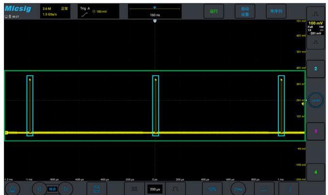
Traditional Single acquisitions can only capture signals continuously, wasted storage depth when testing intermittent signals like laser pulses or serial buses, also difficult to trace back captured events. While the segmented storage acquisition can capture the target signal and allows to play back captured ones, effectively captures target signals multiple times over a long period of time.
