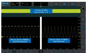
Insufficient memory depth often leads to distortion when long time-base signals were expanded. With memory depth of up to 360Mpts, there is no reduction in performance even with two channels opened at the same time. The signals will still maintain excellent fidelity even at long period of time.
