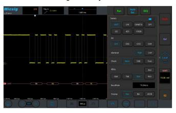
The MHO 3 series standard with 8 serial bus decodes: RS-232/422/485/ UART, CAN, LIN, CAN FD, SPI, I<sup>2</sup>C, ARINC-429, 1553B. With the TXT decoding text mode, the data can be transferred to CSV format.
