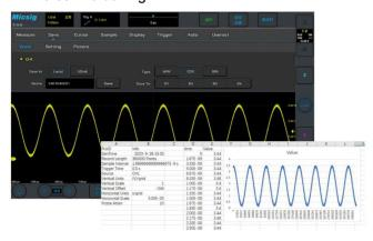
Users can save waveforms and measurement results as binary (BIN) or CSV format files for data analysis using Matlab or Excel. Also support saved as WAV format, open & analysis inside the oscilloscope. Additionally, user can save waveforms as images or record videos.
