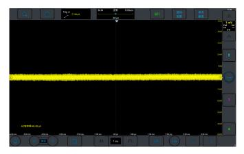
Even at its full bandwidth of 500M, the noise floor of the MHO 3 series still less than  $80\mu Vrms$ , allow engineers accurately capture weak but important signals during daily circuit debugging and signal analysis.
