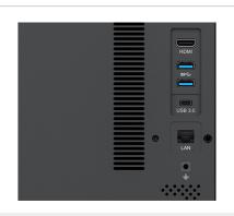
USB 3.0 Host, USB Type-C, LAN, Ground, HDMI, Trigger out and others
