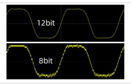
MHO 3 series has 12 bit high-resolution ADC with a quantization level of up to 4096, it's 16 times that of traditional 8-bit ADC, present unmatched waveform details.
