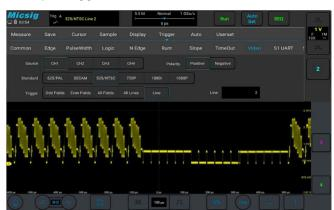
The MHO 3 series provide multiple triggers, including edge, pulse width, logic, Nth edge, Runt, slope, bus decoding, etc. Whether you need to capture specific edge transitions, or observe duration and frequency of the target signal, it meets your requirement at ease.
