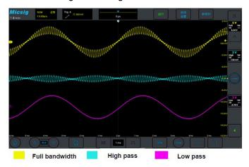
Digital filtering can selectively allow or block signal components within specific frequency ranges.
