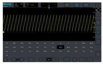
Traditional oscilloscopes need to step in a sequential manner when adjusting the time base. In addition to traditional sequential steps, the MHO 3 series also has a time base matrix, allows user to select any time base in one click.
