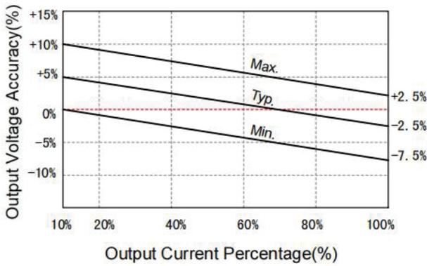
Output Regulation Curve (3.3VDC Output) Figure 1-2
