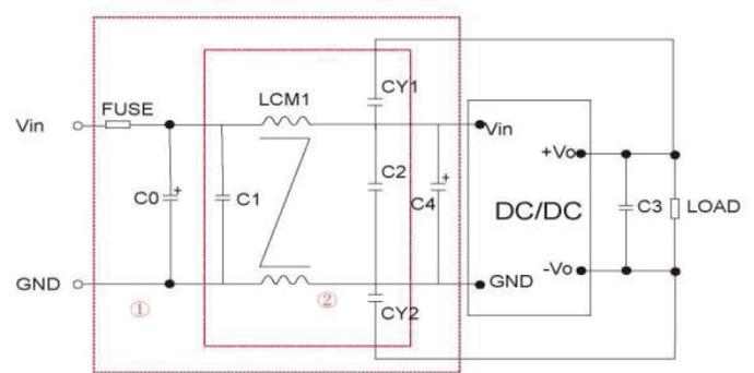
Note: Part ① of Figure 3 is used for EMC testing; Part 2 is used for EMI filtering and can be selected according to requirements.
